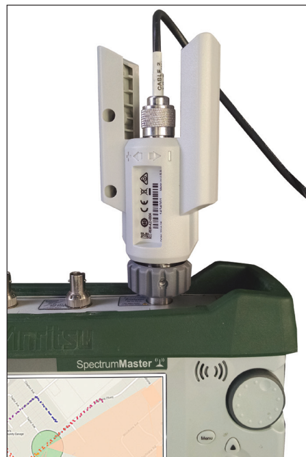
Figure 13: Bandpass filter inserted between spectrum analyzer and RF antenna cable
