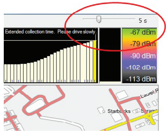
Figure 19: Upper right section of software interface showing position for user to set Max or Min Hold settings (in seconds)
