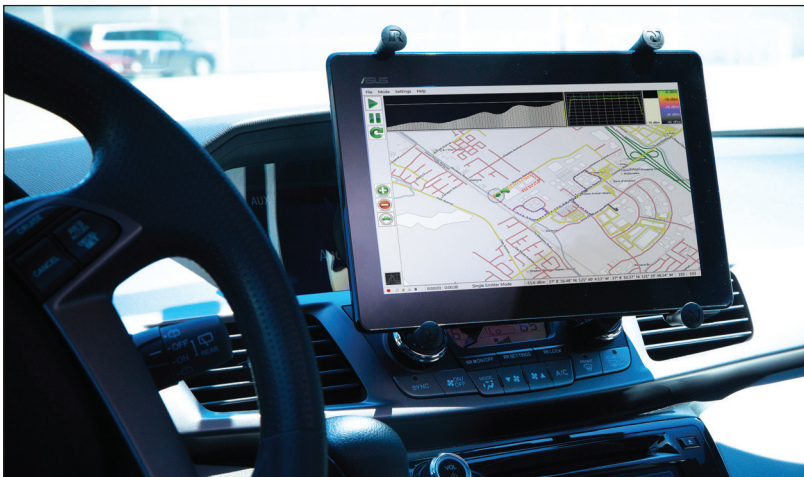
Figure 2: MX280007A Mobile InterferenceHunter™ on Windows PC Tablet with Spectrum Master™ in Vehicle
